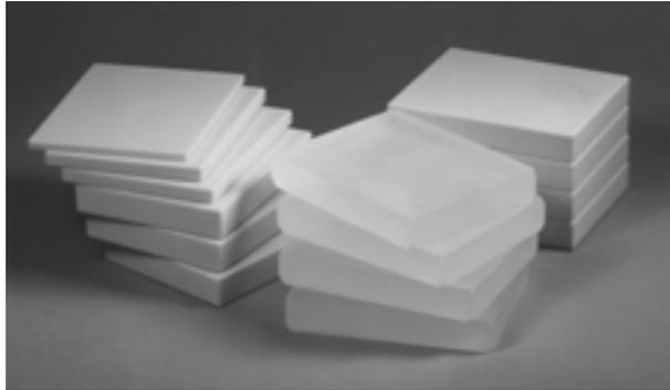
The mammographic unit's automatic exposure control should be capable of maintaining optical density within  $\pm 0.15$  OD as the voltage is varied from 25 to 35 kVp, and as breast thickness is varied from 2 to 8 cm for each technique. Test images taken of uniform phantoms of varying thicknesses should not differ by more than 0.30 OD from each other. These tests should be carried out over the kVp range customarily used by the mammography center.
