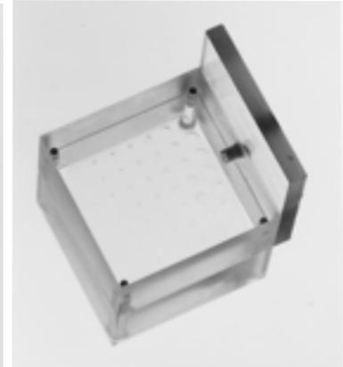
Rotatable support plate accommodates prone-position x-ray units
