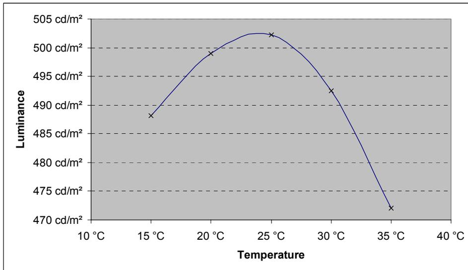
Fig 3: Influence of temperature on the luminance of LCD-based displays
