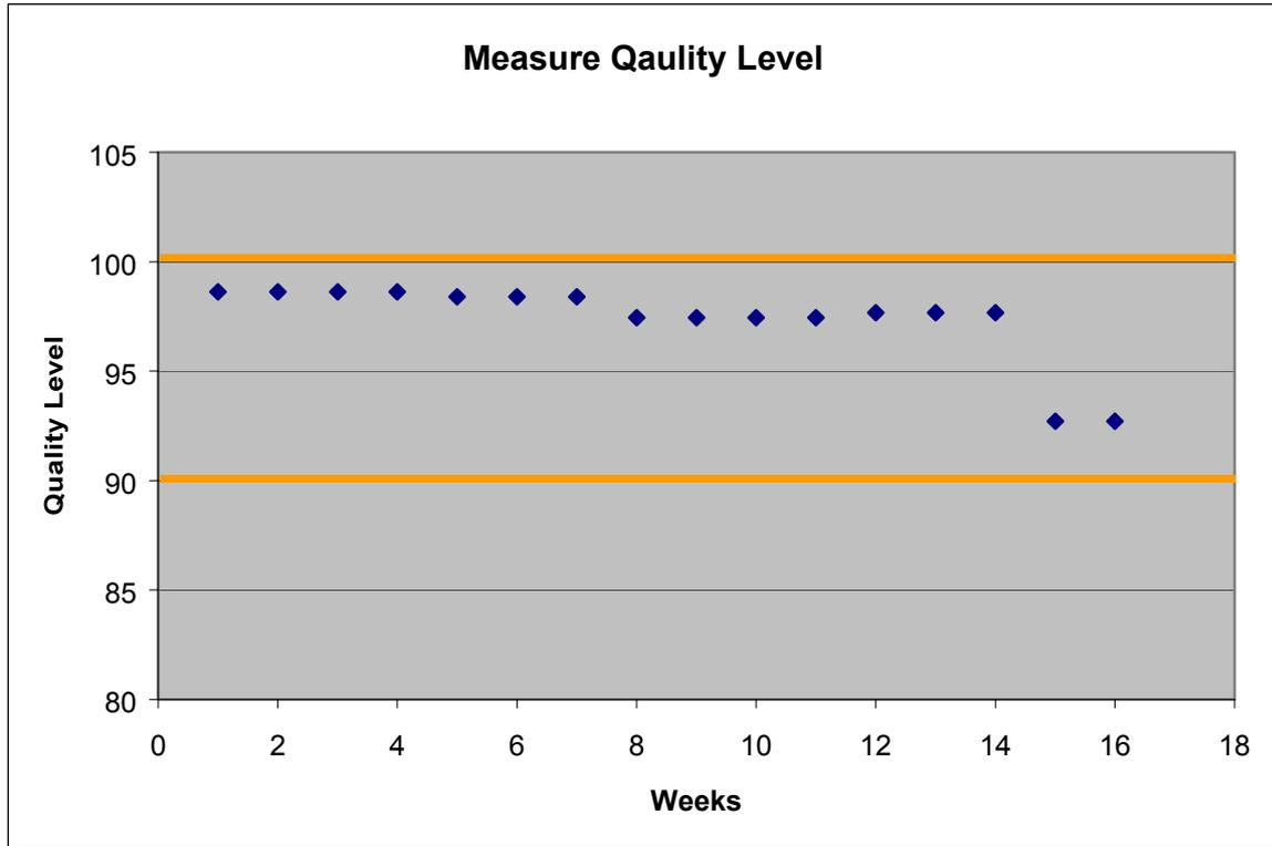
Fig 6: A graph of quality level measurements on a CORONIS display
