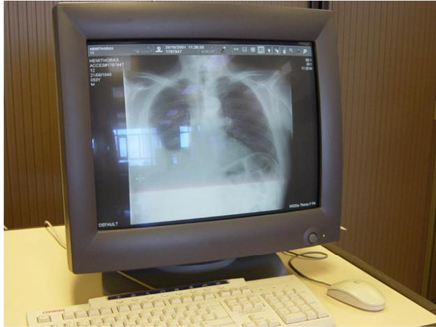
Fig 2: Visual reflection of a window on a CRT based display
