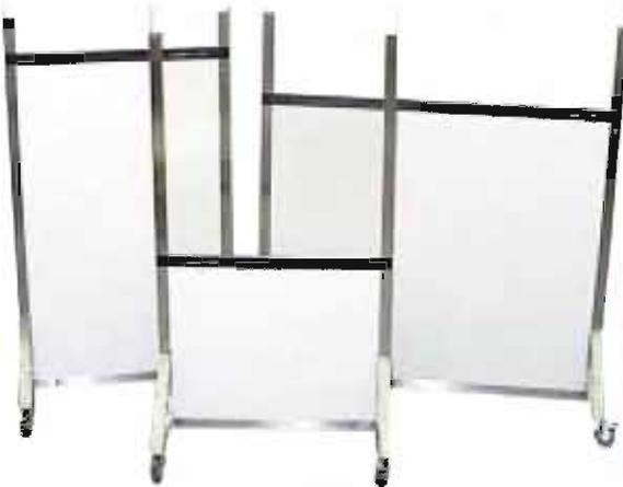
Wolf offers 4 styles of our Non-adjustable Mobile Barriers, (see the table below for the sizes and lead equivalency protections available). Designed with a shatter resistant clear pb viewing area at the top and a white opaque bottom that is also lead lined for your complete protection, the framework is stainless steel with a brushed finish. Casters lock in place for stable positioning.
