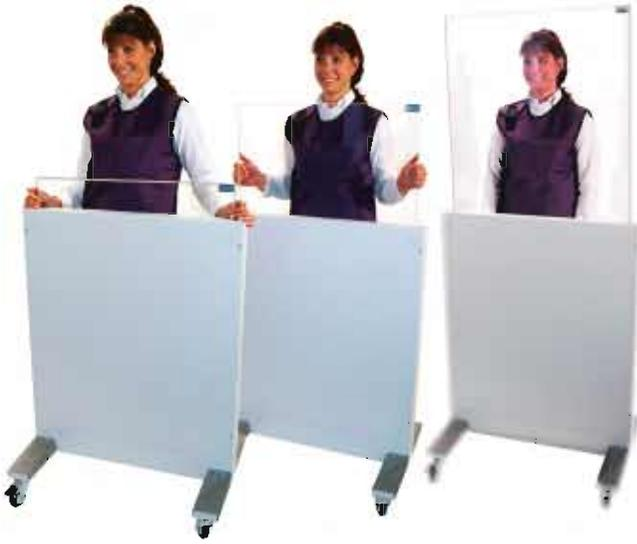
The Adjustable Height Barrier allows the user to position the clear pb at any height level between 45 1/2" and 68". By use of an internal counter-balancing mechanism, the clear pb can be moved up or down with minimal effort.
